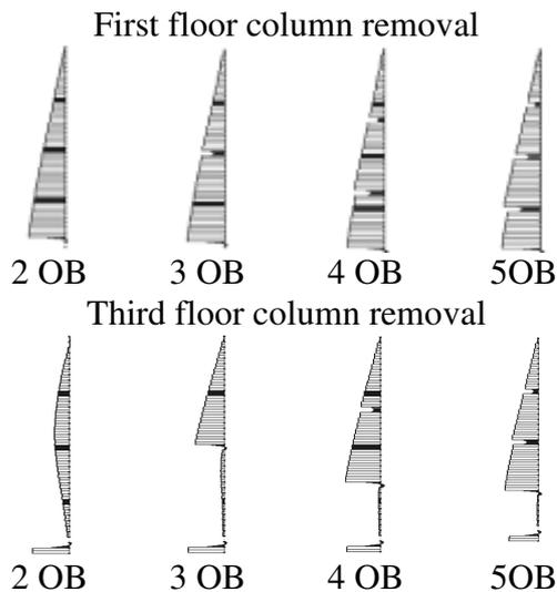
**Fig. 14. Influence of amount of outrigger blocks (OB) on axial force distribution in columns**
