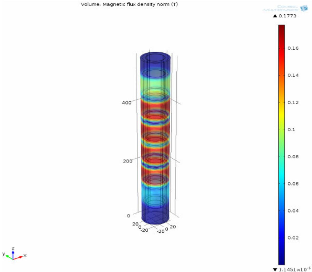
**Picture 10 – 3D model of magnetic induction distribution**
