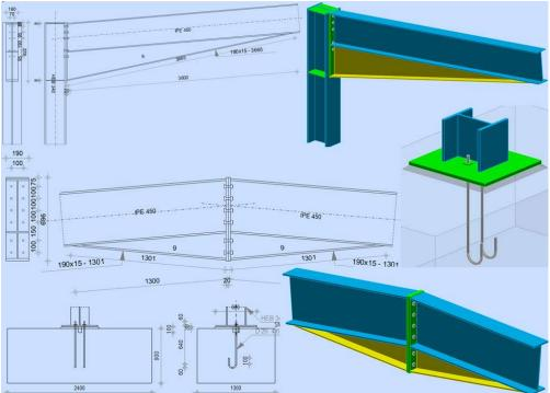
Figure 4 – Design model of the building framework; drawings, spatial view of the main bolted and welded joints
