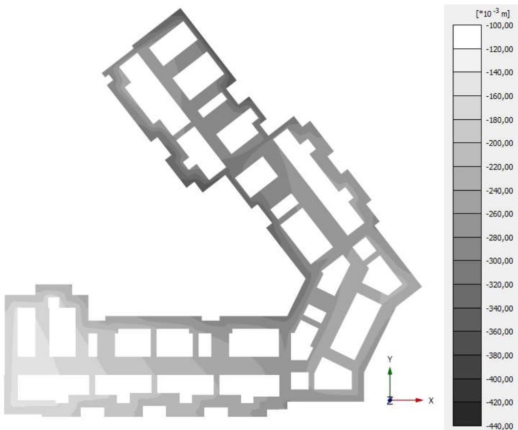
Figure 6 – Results of 3D FEM modeling of the reinforced base of the foundation strip (settlements in mm)
