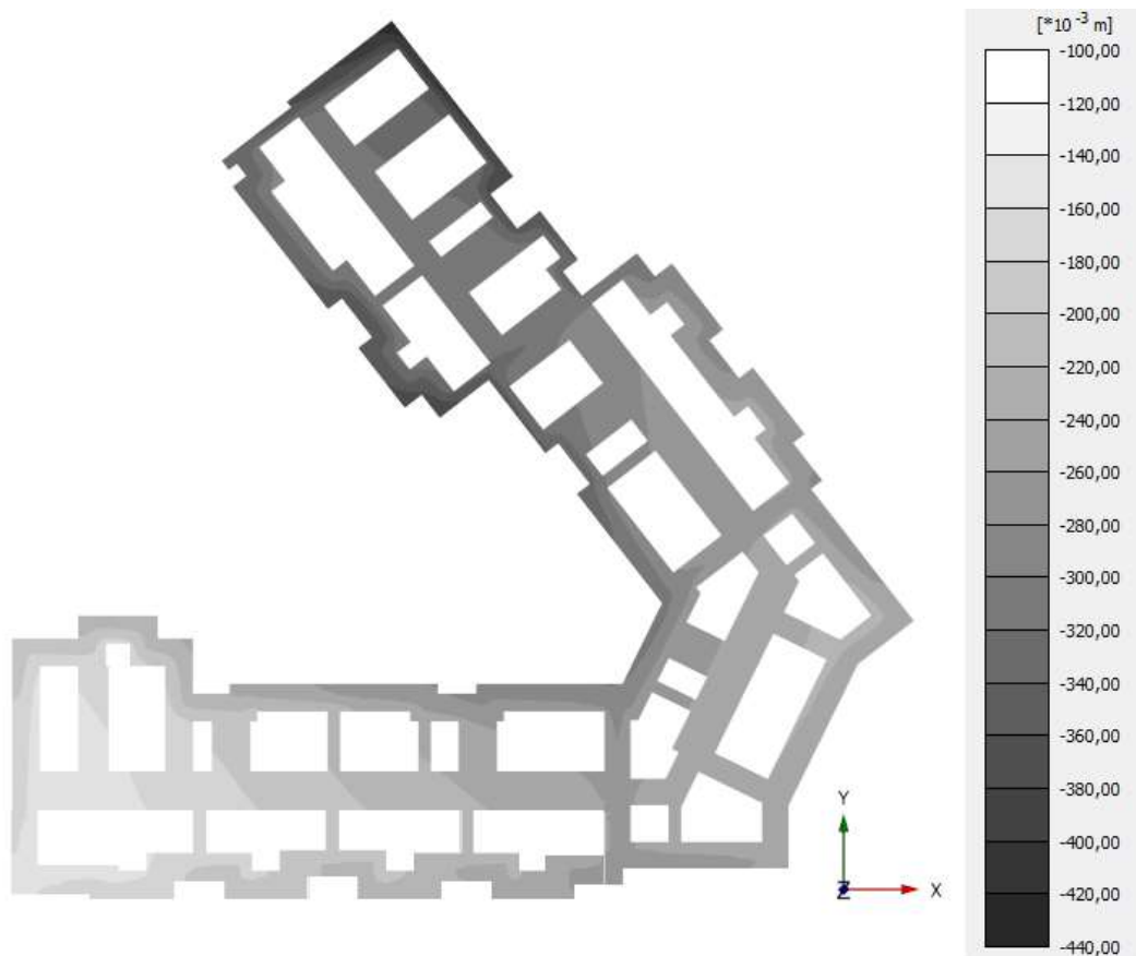
Figure 5 – Results of 3D FEM modeling of the unreinforced base of the foundation strip (settlements in mm)
